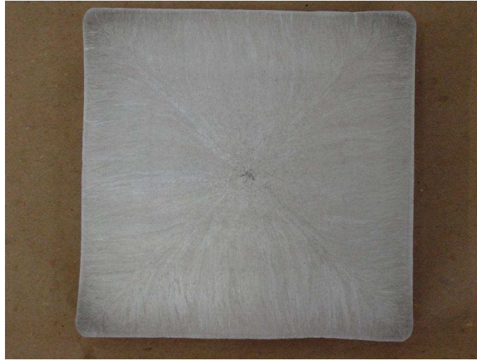
Fig. 6, Macro etch of 304 Stainless steel, casting speed 1.6 m/min
