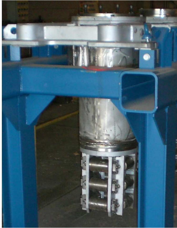
Fig. 4: Particular of mould assembly and billet containment
